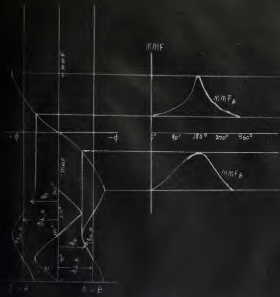
Figure 2 - Projection of Flux onto Saturation Curve to Obtain MMF
